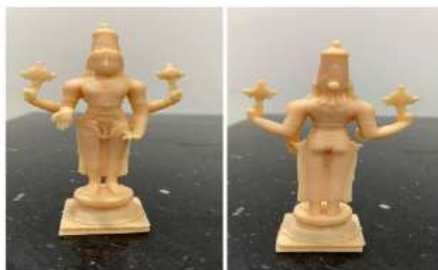
Fig 6. 3D Printed prime model of Srinivasa Perumal statue
