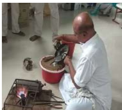
Fig.4.4. Making of lead mould
