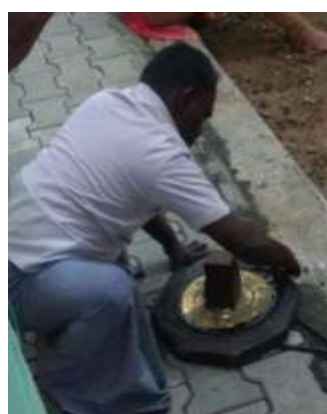
Fig. 4.7 Fixing of brass plate to the wooden base
